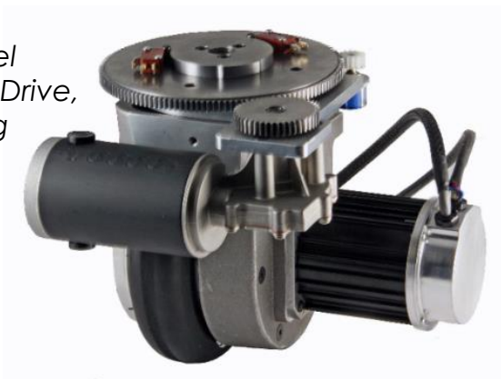
Automated GPS- Guided Vehicle Steering Module with Torque Motor, Integrated Servo Drive with CAN bus
